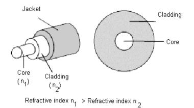
Core is the glass (SiO<sub>2</sub>) area through which light travels and the information is carried
