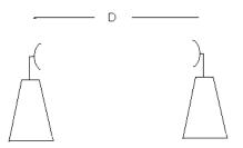
It is a system composed of transmitter and receiver installed on top of two mountains in order to have wireless communication using electromagnetic waves at microwave frequencies. Operates in the UHF (Ultra-High Frequency) up to the EHF (Extremely High Frequency) bands, which covers the range between 300 MHz and 300 GHz, current practice being mainly from 1 GHz up to 45 GHz.
