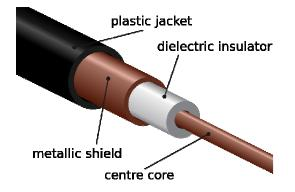
The signal is applied between the centre core (metal) and the metallic shield (ground).
